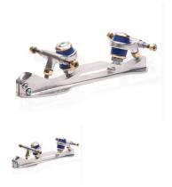
Frame for skaters at a competitive level, aluminum insoles made by milling from right and left solid bars with brake inclination, aluminum crossbars with adjustable steel toe, snap steering adjuster. Elastomer suspensions in 5 hardnesses.
