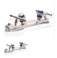
Frame for professional use with light titanium alloy structure and lowered stance with a super elastic and fast mechanical response in the movements of the skate. Right and left insoles made by milling from solid bar, inclined with double brake screw, crosses with axis and adjustable titanium tip that make it lighter. Precision-click steering adjuster with elastomer suspension available in 5 hardnesses.
